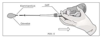
To fire the clip, pull the handle beyond the noticeable resistance.
