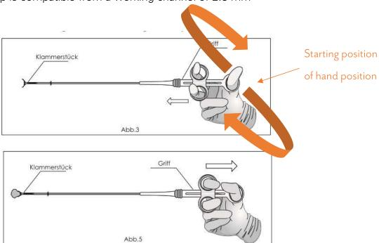
Close the clip by pulling the handle backwards until you feel a noticeable resistance. A new placement is possible by reopening.
