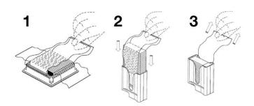
Slides are packed with a special inner wrap to assist with loading into the SlideMate AS hopper to prevent contamination due to handling.
