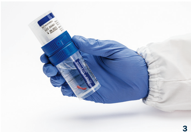
3 Tilt the device and let the formalin flow to the lower container
