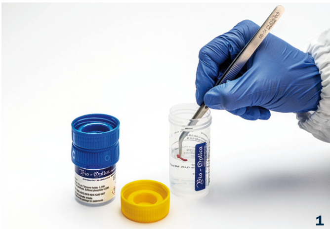
1 Open the container with the yellow lid and release the biopsy into the buffer
