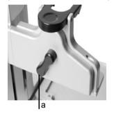
The rear position of the lever (a) moves the pipette to the rear to accommodate the rear positions of 384 well plates.
