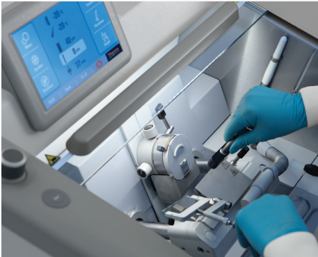
Work chamber is designed for efficient set-up. Removable tray components, an encapsulated microtome, and built-in vacuome aid in quick clean-ups
