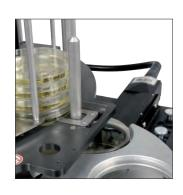
All supported inkjet printers allow side wall imprinting. Alternatively, dishes can be imprinted on the bottom using the LINX 4900 inkjet printer module.
