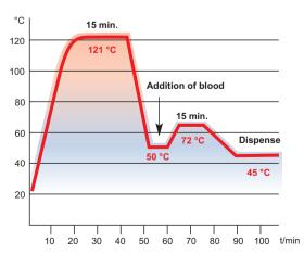
Chocolate Agar mode: After the first sterilization phase, blood is added and again shortly heated up before dispensing.
