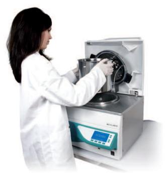
MEDIACLAVE is designed to keep maintenance easy. The absence of any heating element within the sterilization vessel makes the cleaning of the vessel easy.
