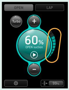
**Activation screen:** The segments on the right-hand side of the screen show the course of the *suction shut-off delay*. The segments on the left-hand side of the screen show the course of the *standby suction time* (not visible in the image).
