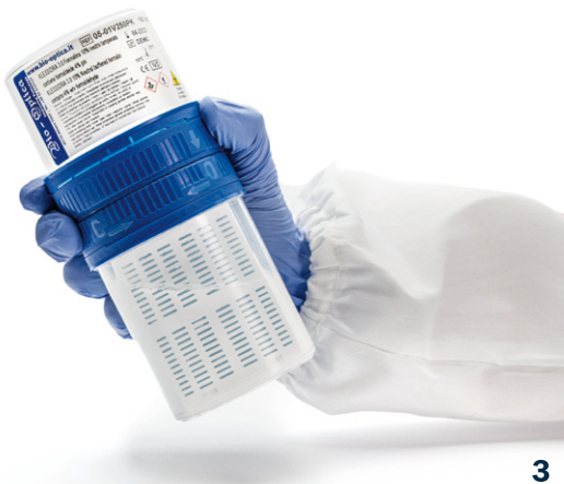
3 Tilt the device and let the formalin flow to the lower container
